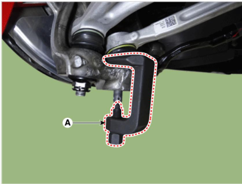
4. Loosen the compression arm pin (A) and nut (B).
