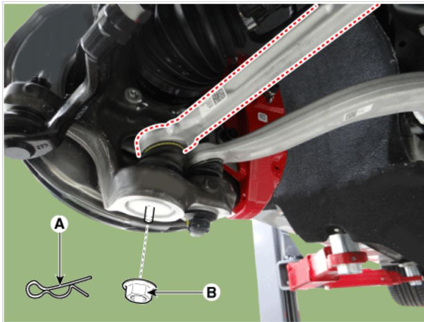
3. Remove the lateral arm by using the ball joint remover (A).
