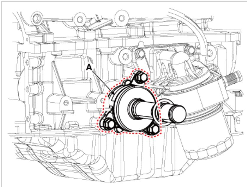
10. Using pry bar (A), separate the front drive shaft from the front differential (B).
