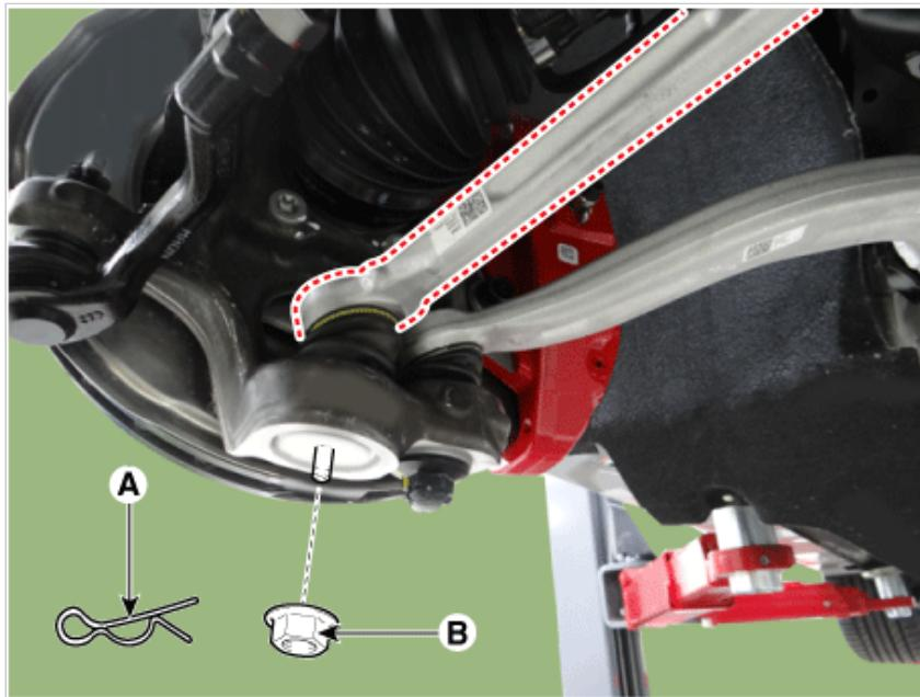
3. Remove the lateral arm by using the ball joint remover (A).
