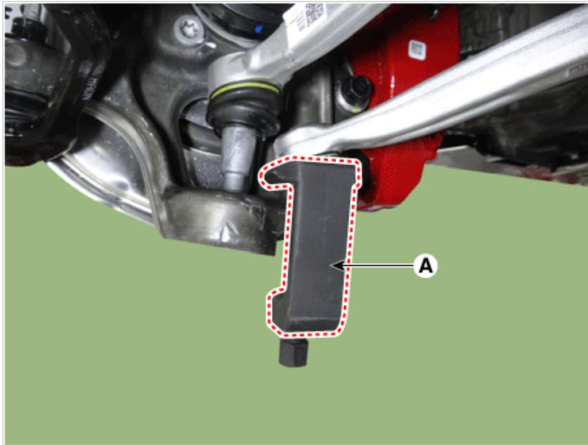
6. Loosen the nut and then separate the stabilizer link from the front shock absorber.
