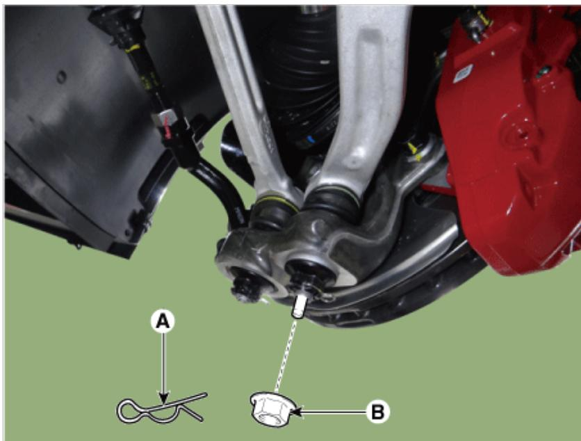
5. Remove the compression arm by using the ball joint remover (A).
