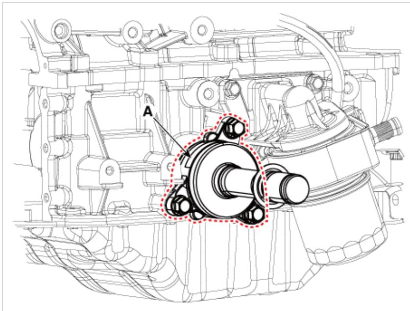
10. Using pry bar (A), separate the front drive shaft from the front differential (B).
